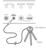
If you have a tripod, use it to place the microphone so that it's about ear level at your normal listening position. If you do not have a tripod, use some other object to install the microphone.
